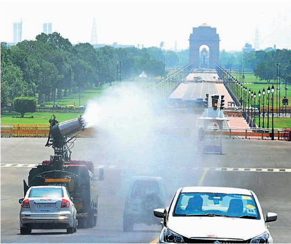
An anti-smog gun on a multi-purpose vehicle sprays water droplets to curb air pollution, at South block on Raisina Hills in New Delhi.
